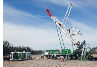
Completions drilling rig in operation
